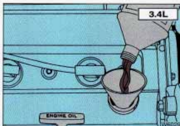
Twin Dual Cam 3.4L V6: Adding Engine Oil
