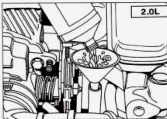
2.0L L4: Adding Automatic Transaxle Fluid
