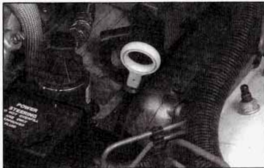
3.8L L36 (Code K) Oil Dipstick Location
