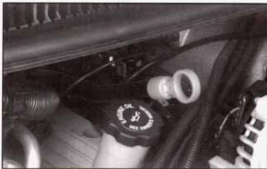
3800 V6 Engine Transmission Dipstick
