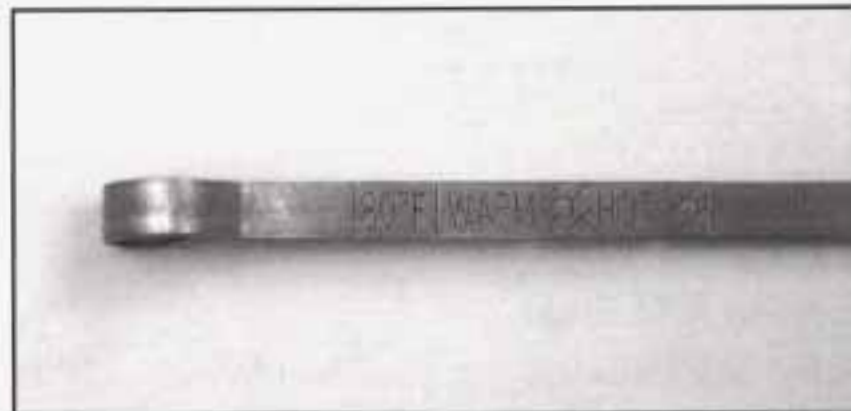
5.7L V8 Engine Transmission Dipstick
