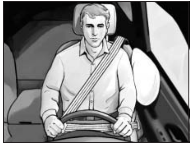
If your vehicle has one, the driver's side impact airbag is in the side of the driver's seatback closest to the door.
