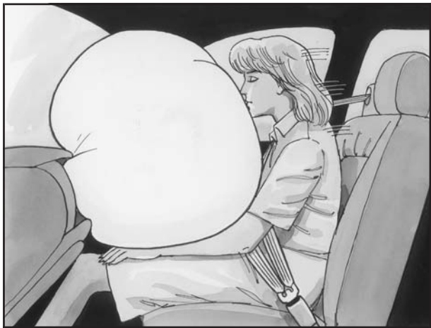
The right front passenger's frontal air bag is in the instrument panel on the passenger's side.
