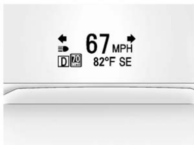
HUD Display on the Vehicle Windshield
