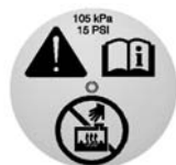
Light-Duty Coolant Surge Tank Pressure Cap
