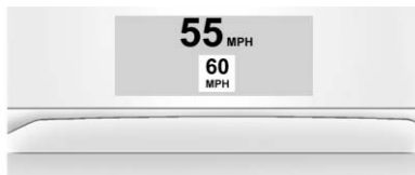
HUD Display on the Vehicle Windshield
