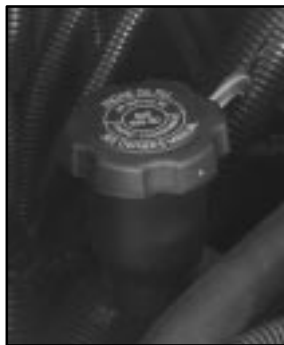
The oil dipstick on the 2200 L4 engine is under the fill cap.
