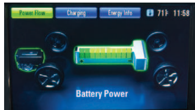
Power Flow screen
